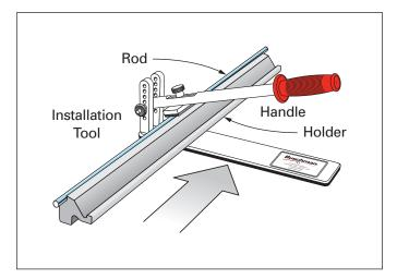
**Step 3:** Slide the installation tool down and repeat until the rod is fully seated for the entire length of the holder.
