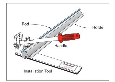
**Step 1:** Starting from one end of the rod holder, place the rod on top of the holder cradle and slide the installation tool underneath.
