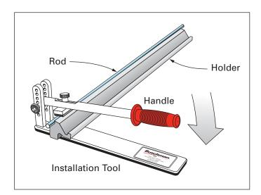
**Step 2:** Press down on the handle until the rod seats in the holder's cradle.
