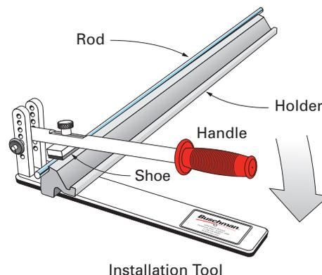
Press down on the handle until the rod seats in the holder's cradle.
